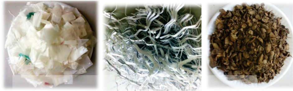
Figure 4.6 The materials used in the RDF-5 preparation: plastics (left), paper (middle) and palm kernels (right).
