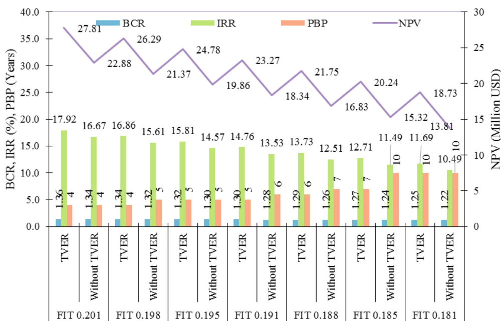
Fig. 16. Variation FIT against the financial indices, with and without T-VER, and for IRR above 10%.
